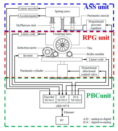
Figure 6. System blocks of quarter-car with the PM-ASS.
