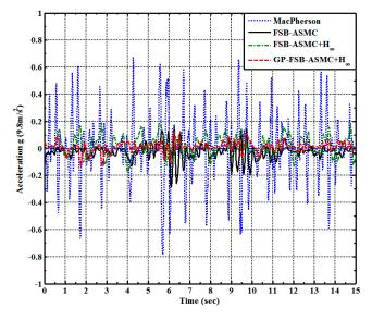
Figure 11. Acceleration of the sprung mass for the rough concave-convex road profile.
