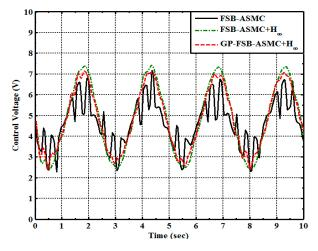
Figure 15. Control voltage for the sine wave excitation road profile.
