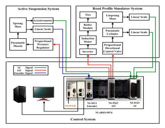
Figure 7. Mechatronics diagram of the quarter-car test-rig with the PM-ASS.
