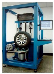
Figure 5. Test-rig of quarter-car using the PM-ASS.
