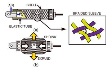
Figure 1. Design of the pneumatic muscle (PM) (a) Components of the PM; (b) Actions of the PM.
