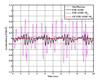
Figure 14. Acceleration of the sprung mass for the sine wave excitation road profile.
