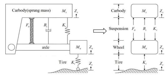
Figure 3. Illustration of a quarter-car with a PM- active suspension system (ASS).
