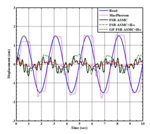
Figure 13. Displacement of the sprung mass for the sine wave excitation road profile.
