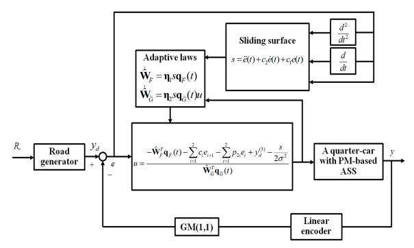
**Figure 4.** Diagram of the overall system for a quarter-car with a PM-ASS that is controlled by the GP-FSB-ASMC+ $H_{\infty}$ .
