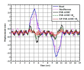
Figure 10. Displacement of the sprung mass for a rough concave-convex road profile.
