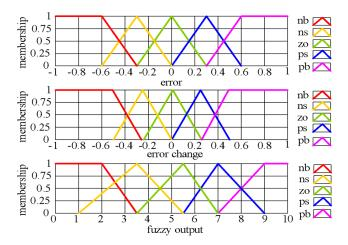
**Figure 9.** Fuzzy partitions and membership functions for the error, the change in error and the fuzzy output.
