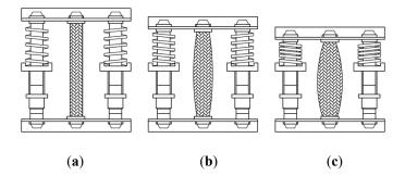
Figure 8. States of the PM (a) no-expansion, (b) half-expanded, (c) fully-expanded.
